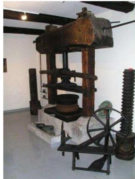
Very old fruit press using screws made of wood.
