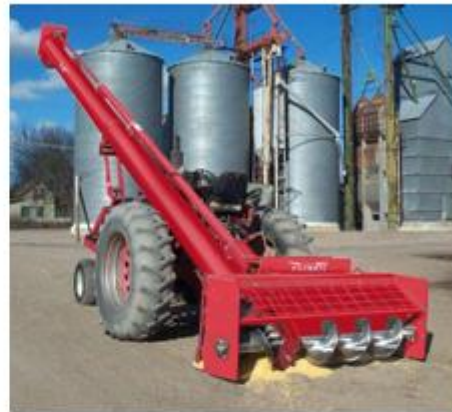
A grain auger used to lift the grain into the storage silo
